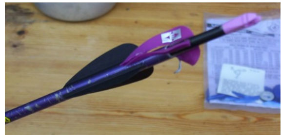
This is the result of a carbon arrow shot from a Compound bow into the back of my wife's aluminium arrow. The carbon arrow went completely inside and only needed new fletchings. The Jazz arrow was trashed.
